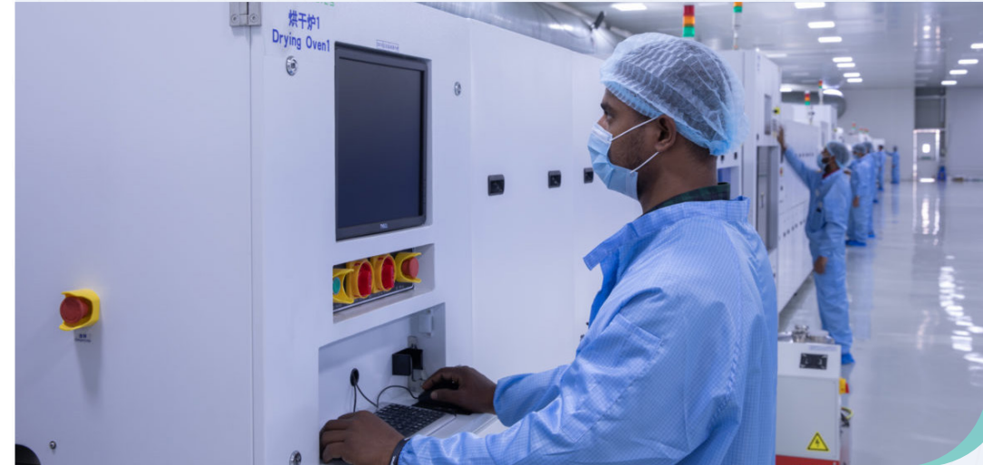
An inline infrared and warm air-drying furnace is utilized for efficient drying of wafers.
